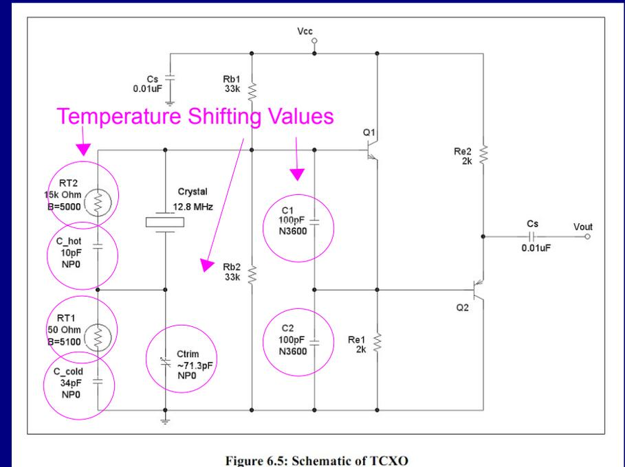
Figure 6.5: Schematic of TCXO
