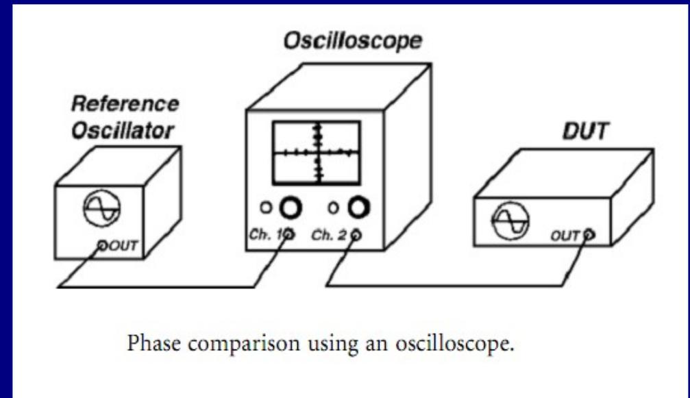
Phase comparison using an oscilloscope.
