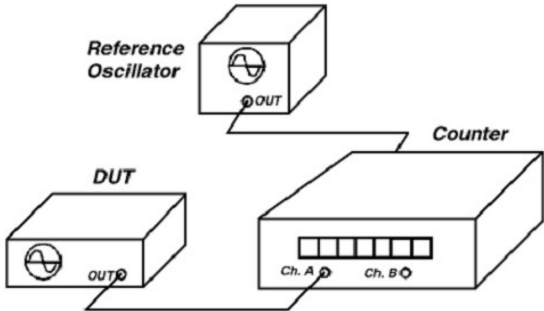
Measurement using a frequency counter.
