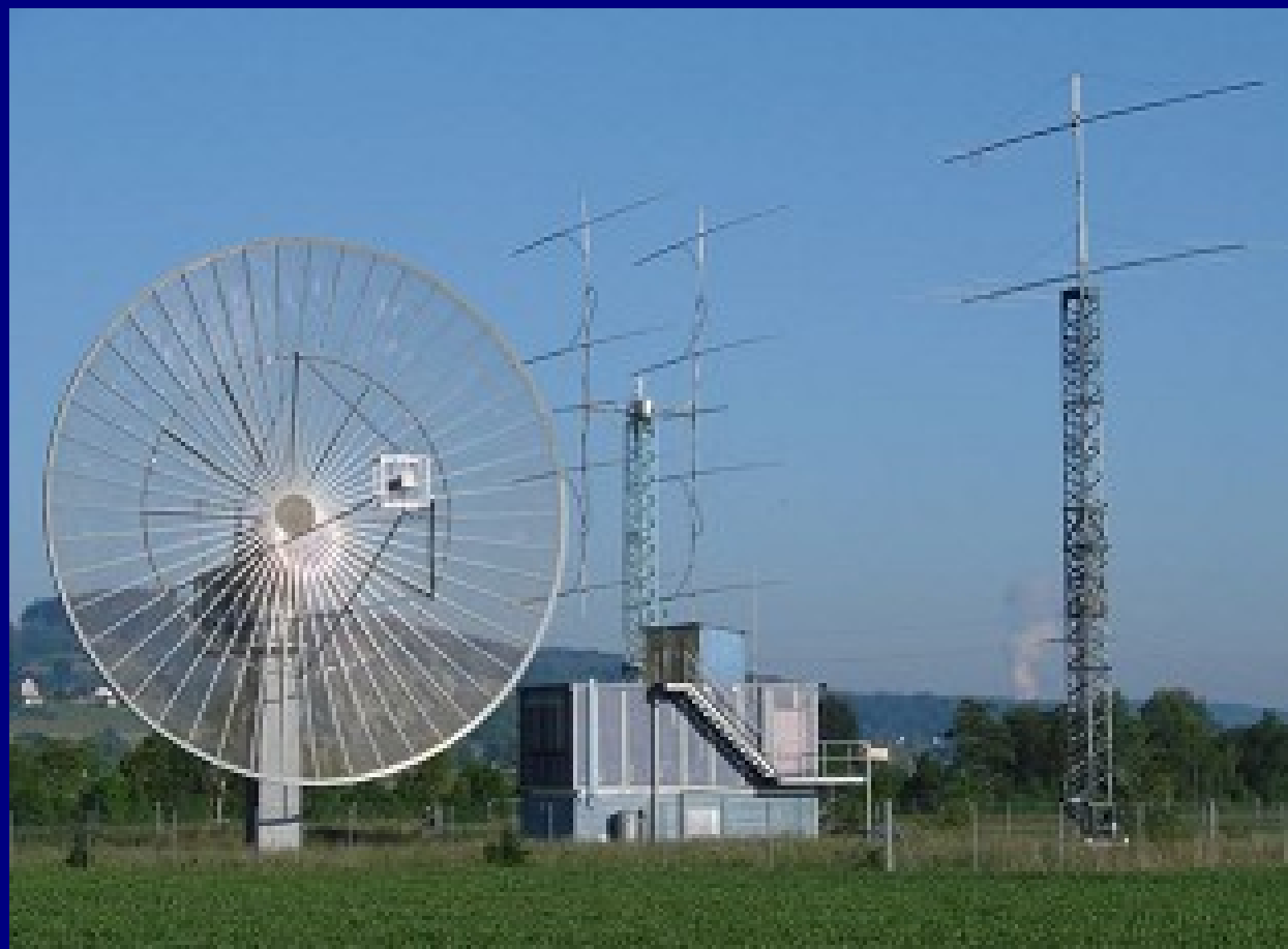
Club HB9Q – Parab.15m (70cm, 23cm, 13cm), 8 x 19 el. Yagis (2m), 11 el. Yagi (6M)
